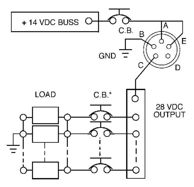
\*THE RATING FOR EACH PROTECTIVE ELEMENT SHOULD TRIP OR RUPTURE IN THE EVENT OF OVERLOAD OR SHORT
